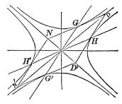
and the tangents ND, N'D' equal and parallel to H'H, the vertices of the parallelogram will fall on the asymptotes.
